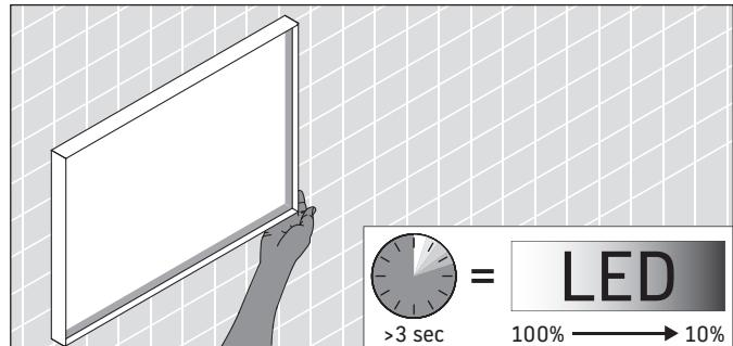
> Hold hand under dimmer for 3+ seconds to dim down light.
