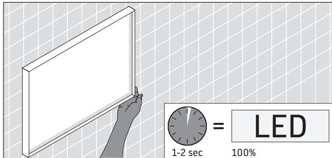
> Hold hand under dimmer sensor for 1-2 seconds for maximum brightness.
