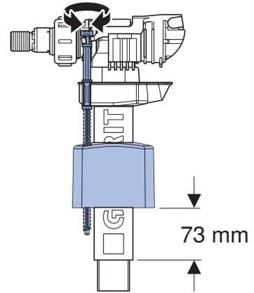
**10** Hook in the fill valve on the lower part of the odour extraction unit.
