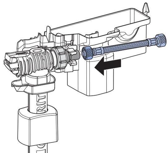
**12** Insert the lower part of the odour extraction unit together with the fill valve.
