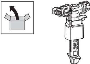
**9** Adjust the fill valve for the correct water level.
